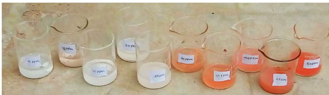
Figure 3.5 Photocatalytic decoloration of Congo Red dye after Sun light radiation (30 min.)
